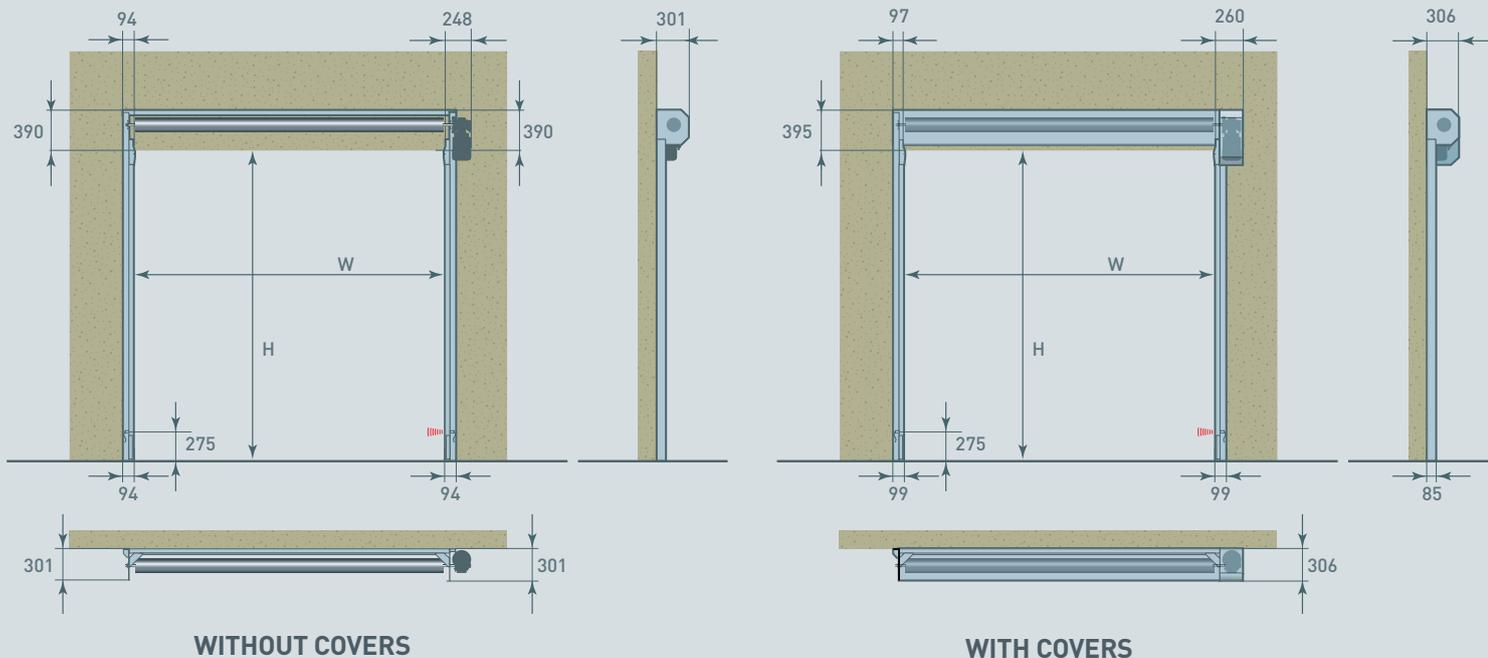
All indicated dimensions are based on exact width and height dimensions only. The space necessary for mounting and maintenance has to be provided.
