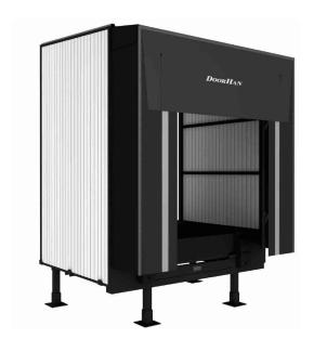
Standard DHOUSH (90/60/45/30) and DHOUST (90/60/45/30) dock houses are used with all types of dock shelters and dock levelers, both with hinged and telescopic lip. Installation time is considerably reduced due to the high degree of pre-assembly of the dock house. At customer's request the dock house may be furnished with cover strips ensuring optimal sealing between the building and dock house.
