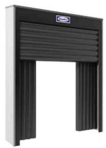
DSHINF inflatable dock shelters provide the best sealing of temperature controlled premises during the loading and unloading. Inflatable cushions cover the truck body around in a way that the optimal sealing is obtained. The cushions are made of high elastic, wear and tear resistant material Cordura. During loading/unloading a part of the truck body is positioned inside the dock shelter. The upper and
