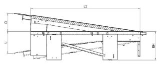
$\begin{array}{ll} BH = profile & O = effective working range above loading bay \\ L2 = platform length & U = effective working range under loading bay \end{array}$
