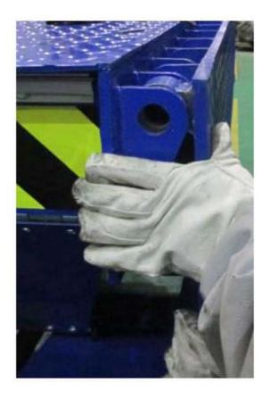
4. Tight the 2nd spring legs with small cables, install on the shaft. Beat the shaft on the other side until the shaft can support all the lips.
