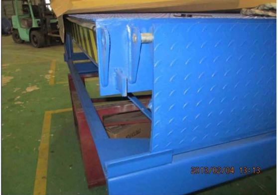
2. For the damaged dock leveler, Weld the bushings on the segment lips that Victor will bring to you as below. Then go to Item 3.
