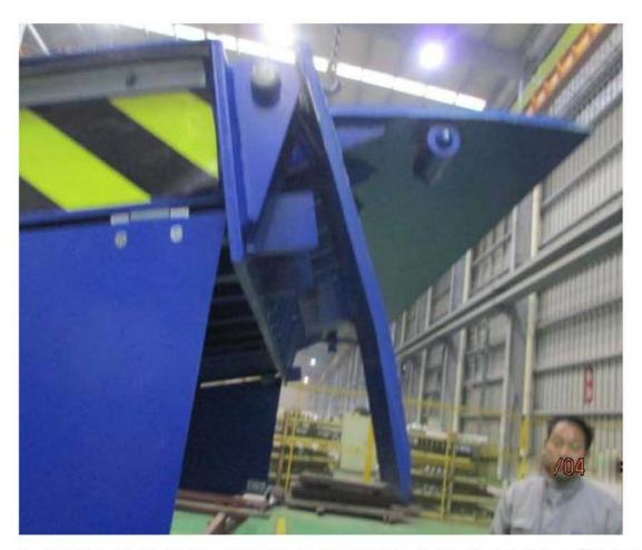
8. In order to move the supports to the center of the dock leveler, Cut the supports of the lips, smooth and install another supports just beside the cut ones. Paint the supports.
